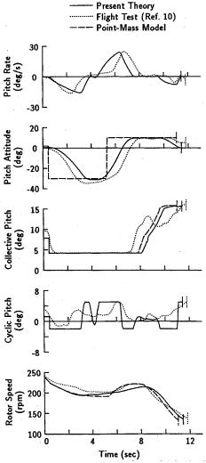
Fig. 10 Comparison of optimal solutions with flight test data<sup>10</sup> for high hover point.
