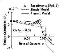
Fig. 6 Necessary torque for a constant thrust in vertical descent.
