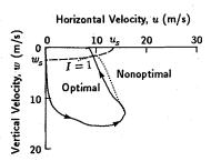
Fig. 11 Comparison of optimal and nonoptimal landing paths from the high hover point.
