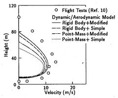
Fig. 7 Effect of dynamic and aerodynamic models on H-V boundary prediction.
