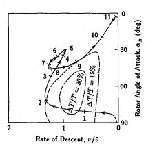
Fig. 13 Locus of optimal solution for the high hover point.
