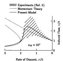
Fig. 4 Induced-flow variation with rate of descent.
