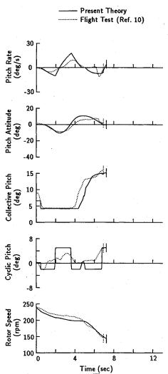
Fig. 14 Comparison of optimal solution with flight test data  $^{10}$  for knee point.
