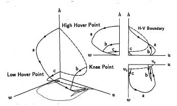
Fig. 9 Loci of optimal landing paths in (h,u,w) space.
