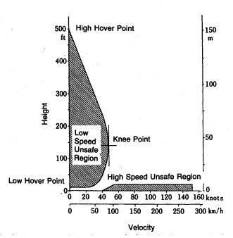
Fig. 2 Typical height-velocity diagram.
