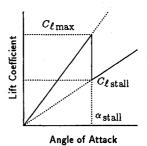
Fig. 5 Lift curve of blade section.
