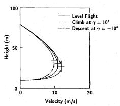
Fig. 8 Effect of initial flight-path angle on the size of unsafe region.
