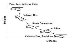
Fig. 1 Autorotative descent and landing following power failure.
