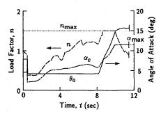
Fig. 12 Time histories of the optimal solution for the high hover point.
